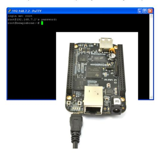
The BeagleBone Black is being pitched as an American (Raspberry) Pi. It has a similar feature set, including video output. However, where as the Pi is intended as a general purpose Linux machine, the BBB (as we shall call it here) is much better equipped for connecting to external electronics, with many more GPIO pins, analog inputs and fast booting into Ångström Linux.
